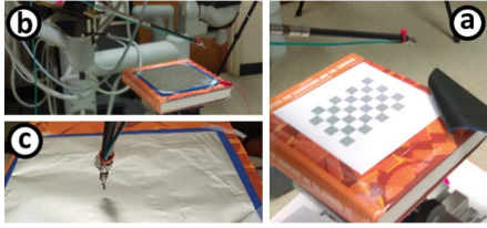
Fig. 10. Experimental test setup. (a) Board is placed under the endoscope to detect the corners. Carbon paper is placed on the board to record the X - and Y -error components. (b) Conductive foil is then placed on top to record the Z -axis error. (c) Manipulator is set to touch to the board corners.
